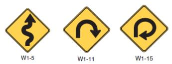
Curve warning sign usage depends on the roadway geometry of the first curve, the advisory speed of the sharpest corner, and whether it is a single curve or multiple curves. Alignment warning signs may be placed a maximum distance of 100 feet in advance of the curve, and a minimum distance of 100 feet from any other signs.
