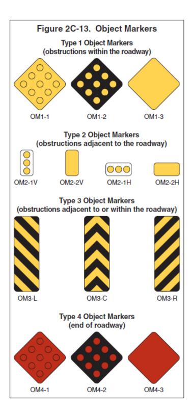
*MUTCD Sections 2C.63 to 2C.65* provide detailed information about the use and installation of object markers.
