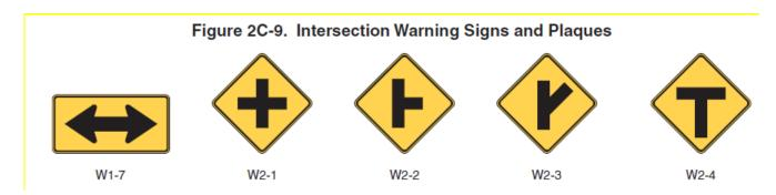
*Combination horizontal alignment/intersection signs* are used at intersections where side roads intersect a main road. These may be appropriate for locations where separate signs for intersections or curves might be misleading.
