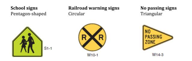
Effective warning signs can reduce incidents by improving driver Perception-Response Times (PRT). A standard PRT value is typically **2.5 seconds** (with 2.5 to 3.0 seconds for older drivers, and longer times for unexpected events).
